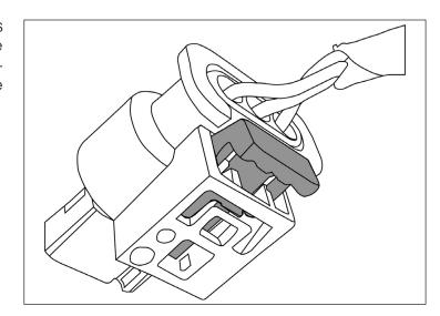
3. Once all conectors are disconnected, use a flat-blade screwdriver to pop all the harness fasteners off the bumper. Remove the harness and set aside. Label each sensor on the OE bumper (outer left, inner left, inner right, outer right) with a sharpie or by other means.
