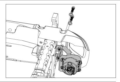
10. Position Tube Overrider and Rubber Spacer to align with Overrider Mounting Bracket and Bumper Shell. Using supplied M10 Nut and Washer, loosely attach Overrider.
